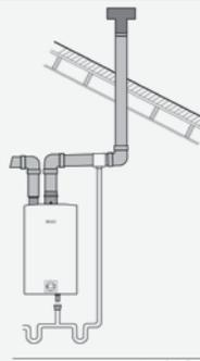
**Exterior Air Intake: Sealed Combustion**
