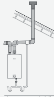
Room Air Intake: Vertical
